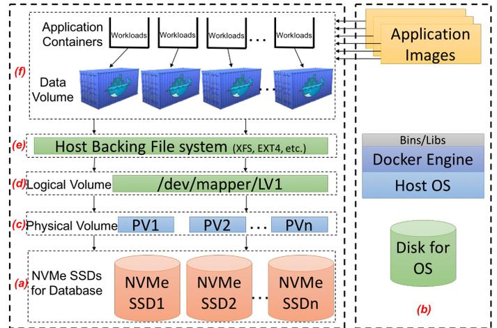
Fig. 1. Containerized system on flash volume of SSDs
