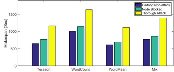
Fig. 4: Makespan without any attack: (1) Hadoop:Non-attack (Native Hadoop) (2) Node Blocked (Native Hadoop with one nodeManager blocked), and (3) with thorough attack.
