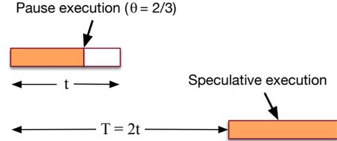
Fig. 1: Intuitions of the attack: In this example, the attacker pauses the execution of a task when it reaches the progress of  $\frac{2}{3}$ . The Hadoop system waits until time  $T = 2 \cdot t$  to realize that it is worthwhile to start a speculative task. At time  $T$ , the original task is expected to be finished at  $\frac{T}{\theta} = \frac{3}{2} \cdot T = 3 \cdot t$ , which is the same as starting a speculative task ( $T + t = 3 \cdot t$ ).
